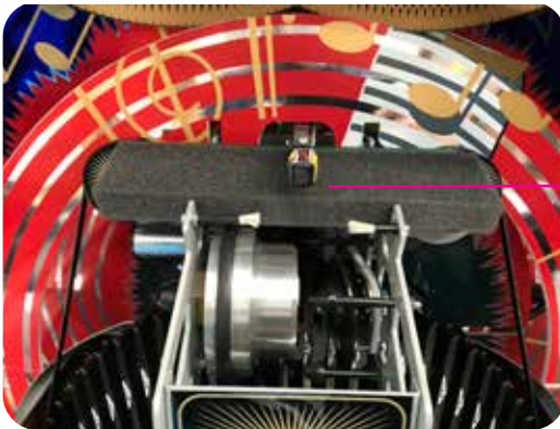
FIG2 : Mechanism in transit mode showing retaining foam
