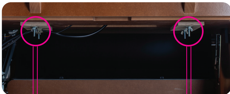
Mechanism retaining wingnuts (underside)
