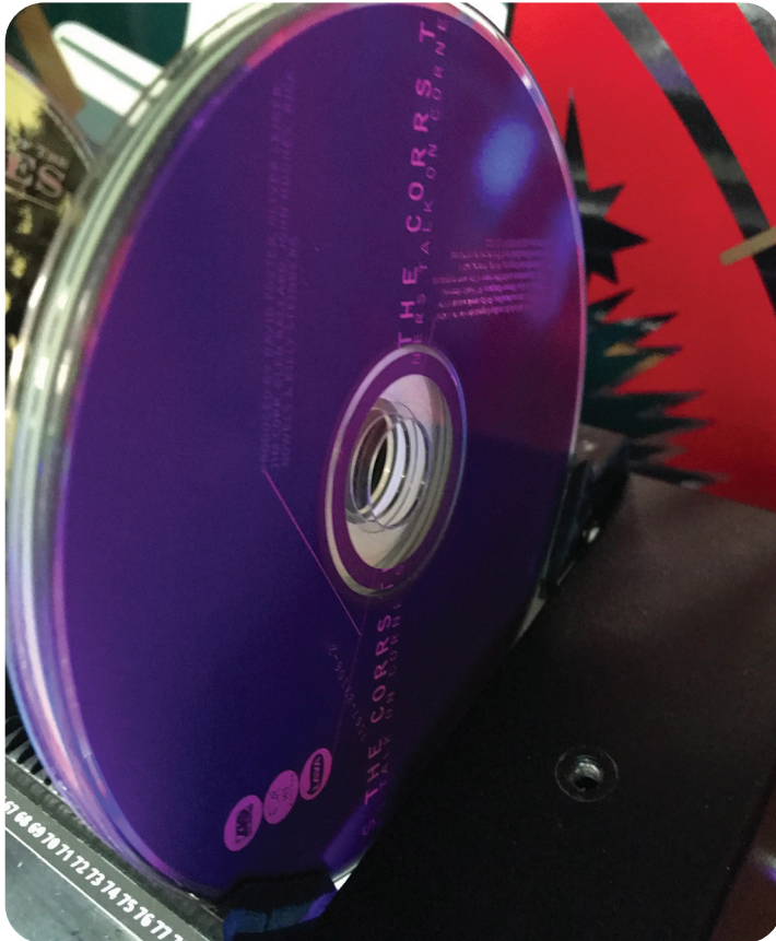
FIG4 : CDs inserted into the mechanism Note the printed side is facing towards the right
