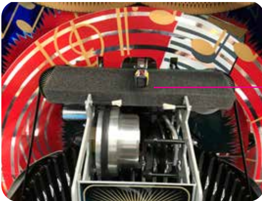
FIG2 : Mechanism in transit mode showing retaining foam
