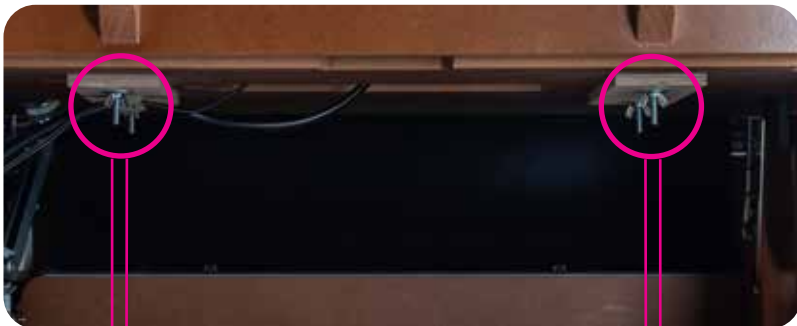
Mechanism retaining wingnuts (underside)
